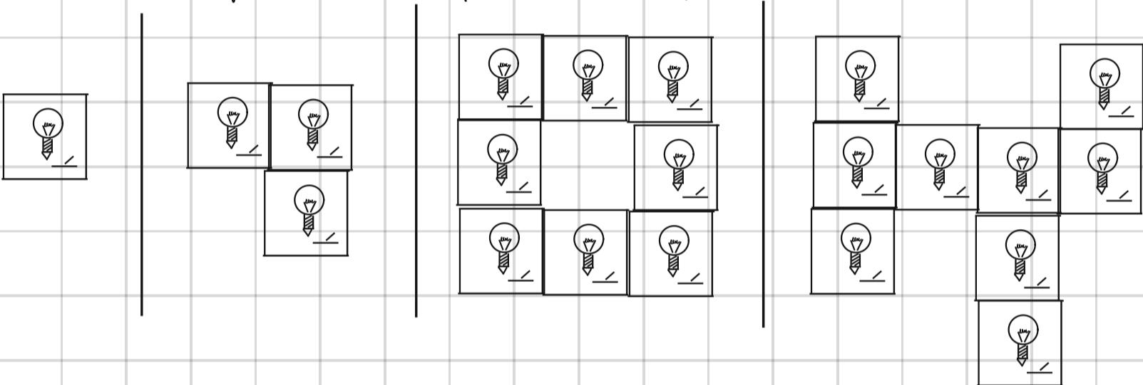
Each switch controls the lamp in its own box and the lamps in boxes that share a wall with its box. Thus, if we activate the switch in the central box, the following occurs:
